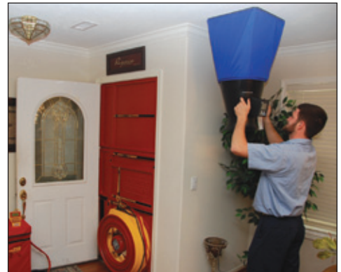
We use a blower door and an airflow capture hood to measure air pressure and air flow.
